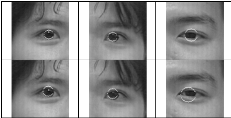
Fig. 6. Pupil features extracted by the proposed MHT (upper row) and the RWHT [19] (lower row).
