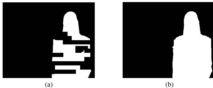
Fig. 7. The simulation results without (a) and with (b) application of the proposed shape recovery approach to the 9th VOP of the “Weather” sequence with BER = 0.05\% and N_{ave} = 4 .
