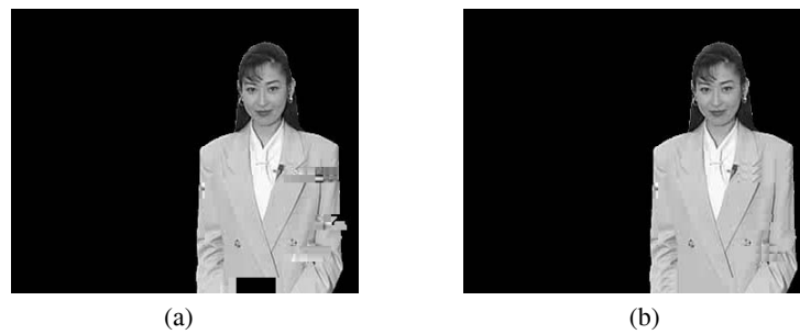
Fig. 10. The simulation results obtained when the proposed detection and concealment approach is applied without (a) and with (b) the backtracking procedure to the first VOP of the “Weather” sequence with BER = 0.05\% and N_{ave} = 4 .
