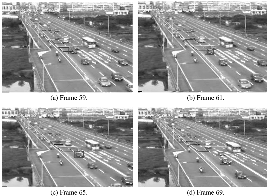
Fig. 15. Our tracking algorithm is able to track a vehicle that performs a lane change.
