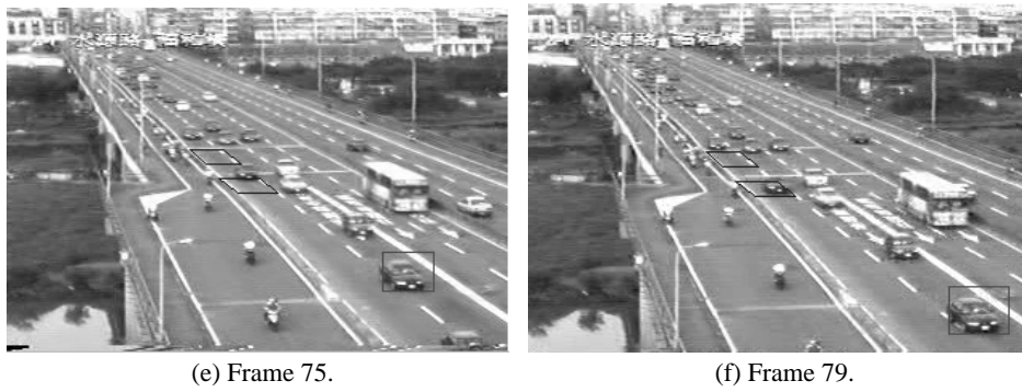
Fig. 15. (Cont'd) Our tracking algorithm is able to track a vehicle that performs a lane change.
