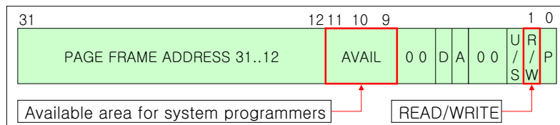
Fig. 1. Page table entry in the i386 version of the Linux Kernel.
