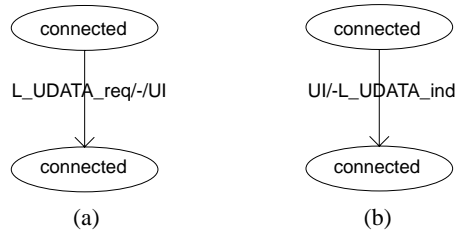
Fig. 6. User information transfer using unconfirmed sender and unconfirmed receiver .
