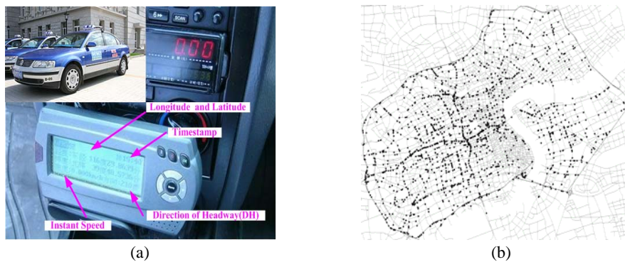
Fig. 2. (a) GPS-based sensor deployed on the dash board of a taxi; (b) Visualization of SUVSNet (The surrounded area depicts the inner-loop area, every dot represents a taxi).
