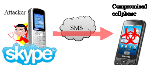
Fig. 2. Command delivery phase of a MAC-YURI attack.
