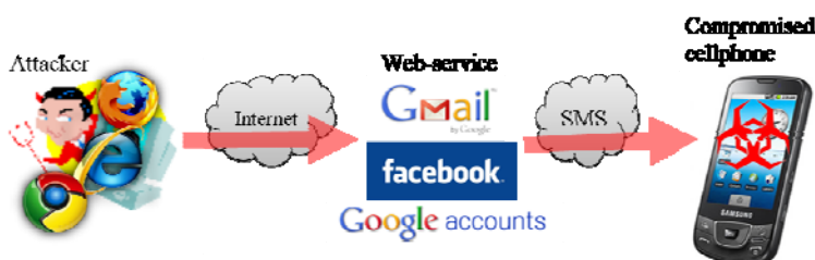
Fig. 3. Verification code delivery phase of a MAC-YURI attack.
