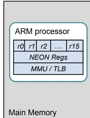
**Figure 2.2:** An example of the ARM virtual processor.
