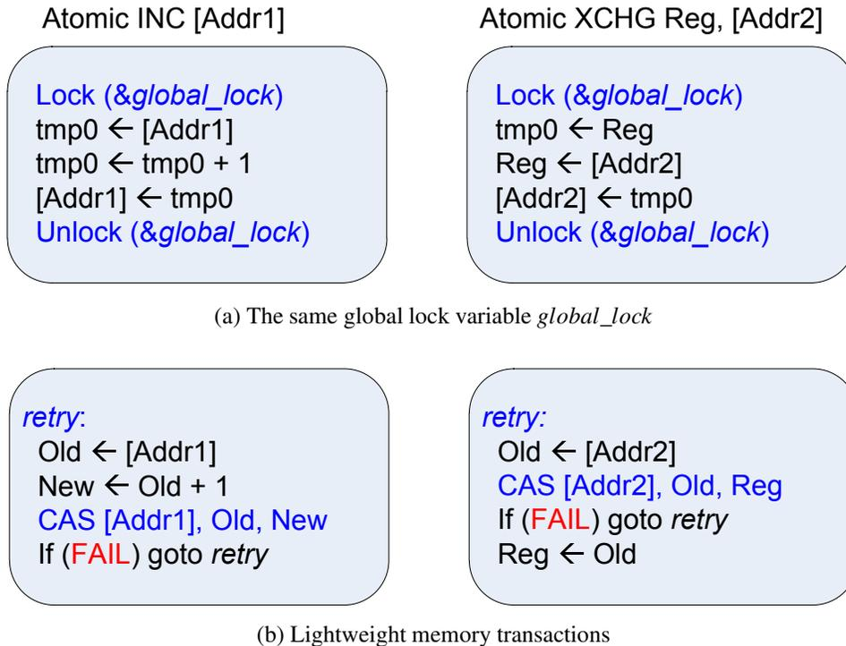
**Figure 5.3:** An example of translating two atomic instructions using (a) global lock and (b) lightweight memory transactions. QEMU uses the same global lock variable surrounding the translated code region of all guest atomic instructions. HQEMU uses lightweight memory transactions to provide the atomic region for all such critical sections.
