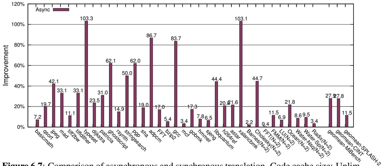
**Figure 6.7:** Comparison of asynchronous and synchronous translation. Code cache size: Unlimited. (baseline = Synchronous translation)
