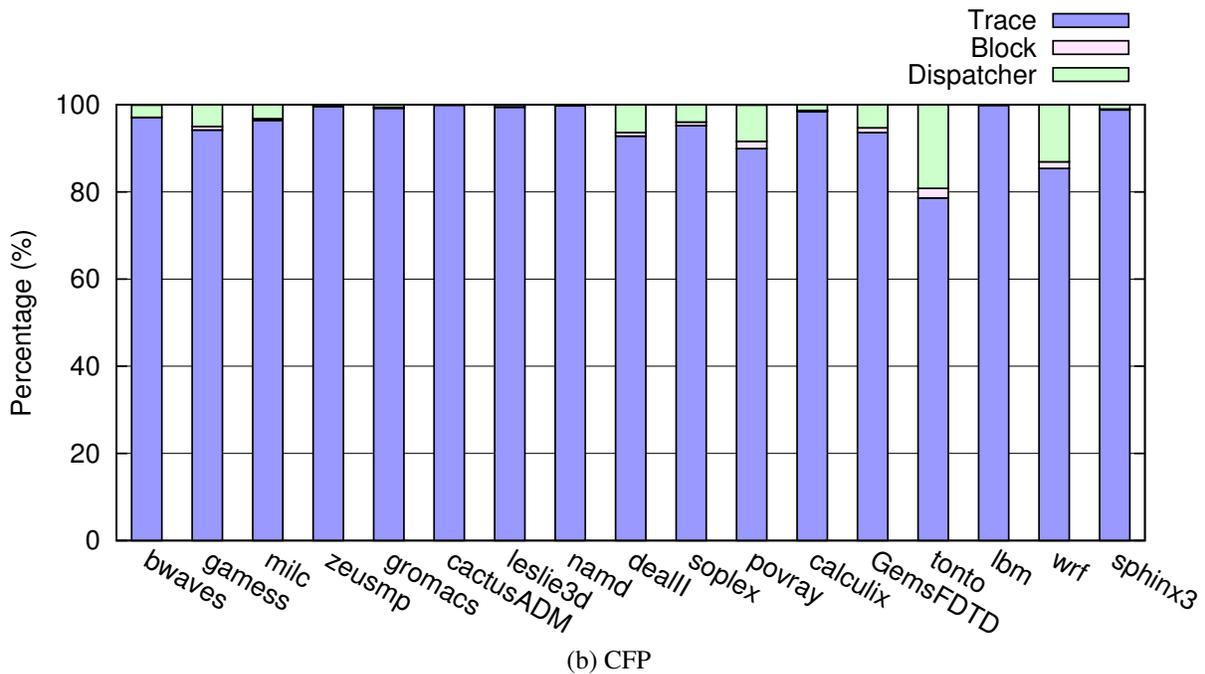
**Figure 3.14:** Breakdown of time with x86 to x86-64 emulation for SPEC CPU2006 benchmarks with reference input. The results show that the execution is mostly within the trace cache—the optimized code from the LLVM translator is effectively utilized by the emulation thread most of the time.
