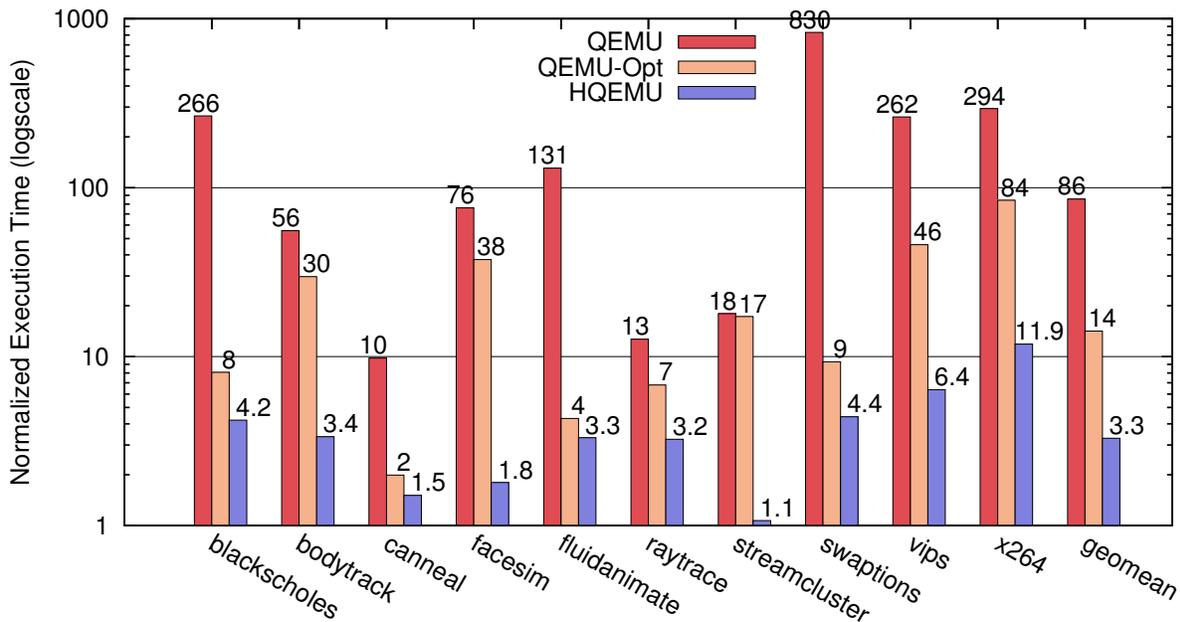
**Figure 5.5:** PARSEC results of x86 to x86-64 emulation with 32 threads and native input sets. Y-axis shows the normalized execution time over native run in logscale.
