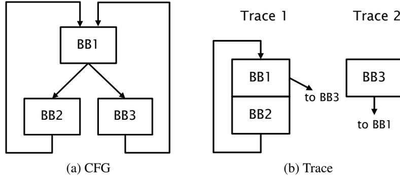
**Figure 3.4:** A CFG of three basic blocks and traces generated with NET trace selection algorithm. Since NET can only form traces of straight fall-through path or simple loop, two separate traces are formed in (b) for the two-loop CFG in (a).
