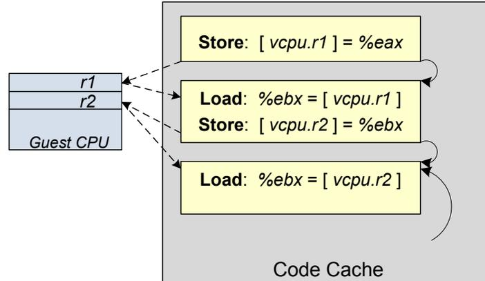
**Figure 2.4:** A code region transition example. During region transition, the states are synced to the virtual CPU when leaving a region and reloaded at the next region. Each box in the code cache represents a code region. A solid-line arrow represents a transition and a dash-line arrow represents a memory load/store operation from/to the guest CPU.
