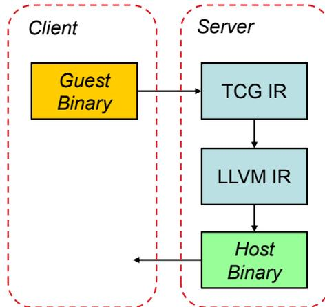
**Figure 6.2:** Two-level IR conversion in the distributed DBT system.
