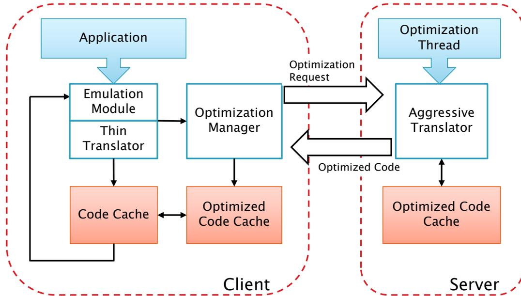
**Figure 6.1:** The architecture of the distributed DBT system.
