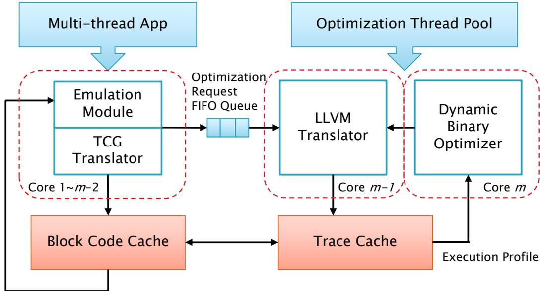
**Figure 3.2:** The architecture of HQEMU on an  $m$ -core platform.
