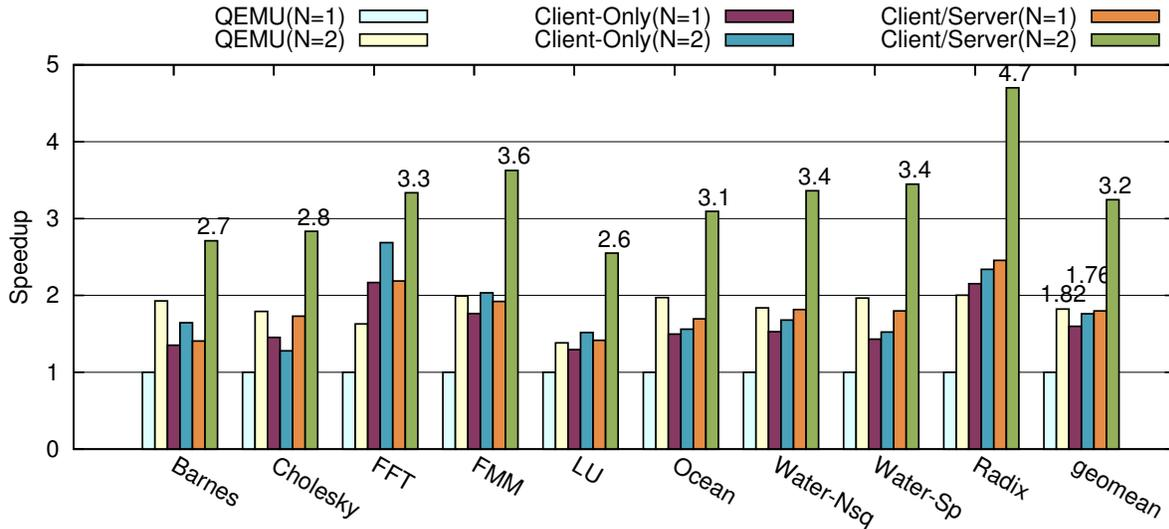
**Figure 6.6:** SPLASH-2 results of x86-32 to ARM emulation with large data sets.  $N$  represents the number of emulation thread. Code cache size: Unlimited.
