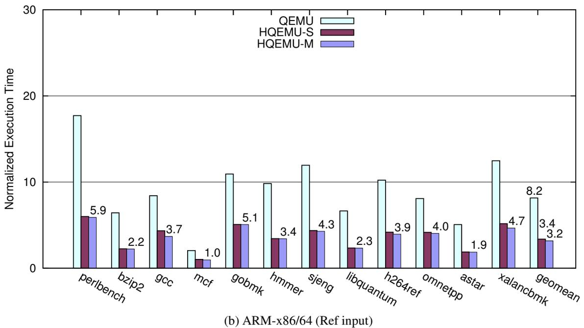
**Figure 3.9:** CINT2006 results of ARM-x86/64 emulation with test and reference inputs. Y-axis shows the normalized execution time over native run.
