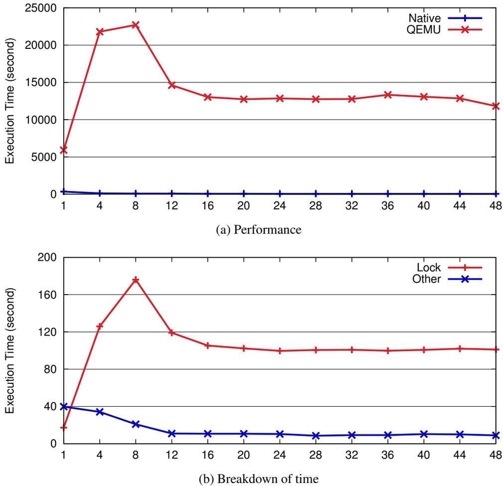
**Figure 2.6:** (a) blackscholes result of x86-32 to x86-64 emulation with native input. The results show that the scalability of QEMU is poor. (b) Breakdown of time with simlarge input. X-axis shows the number of threads, and the unit of time for Y-axis is in seconds.
