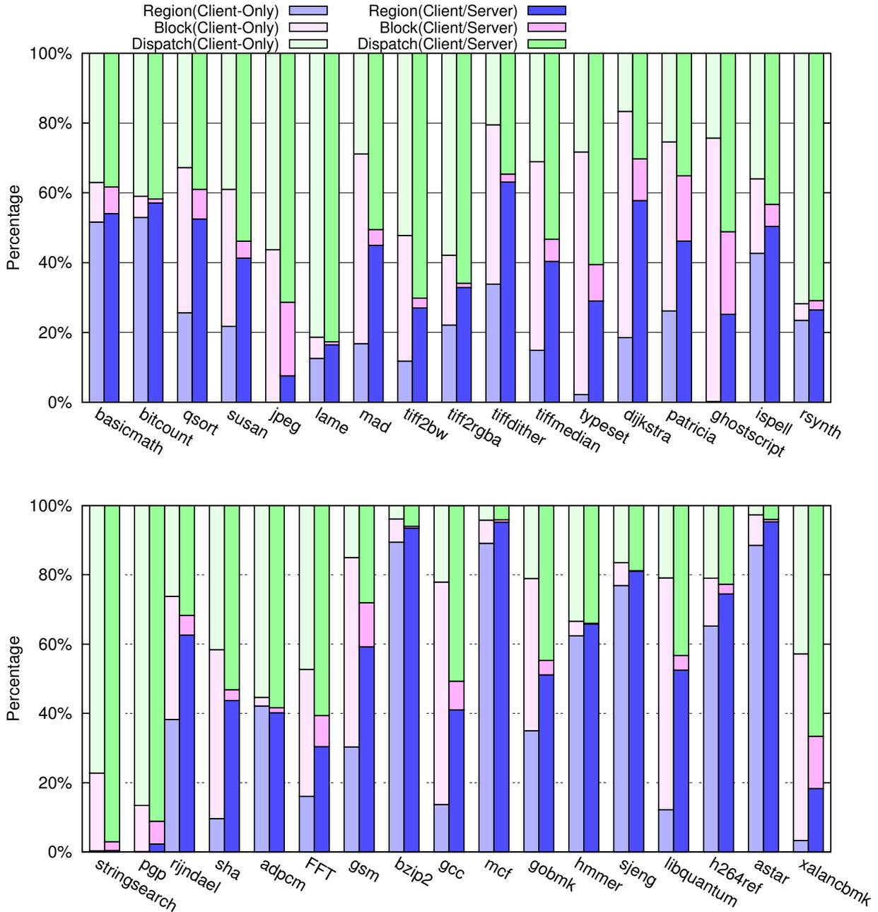
**Figure 6.5:** Breakdown of time of x86-32 to ARM emulation for MiBench with large inputs and CINT2006 with test inputs comparing Client-Only and Client/Server mode.
