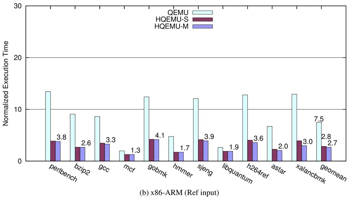
**Figure 3.11:** CINT2006 results of x86/32-ARM emulation with test and reference inputs. Y-axis shows the normalized execution time over native run.
