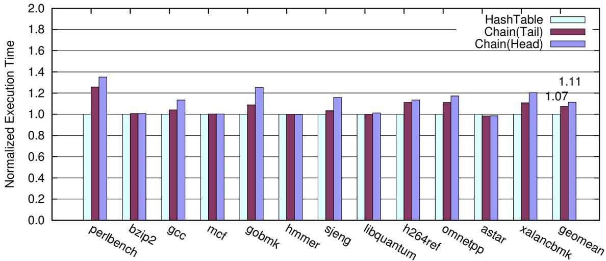
**Figure 5.2:** Performance comparison of Pin’s indirect branch chain with IBTC hash table for CINT2006 with reference inputs. Tail and Head refer to attaching a new chain entry to the tail or head of the chain list, respectively. Y-axis shows the normalized execution time over using IBTC hash table.
