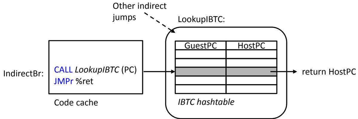
**Figure 5.1:** Implementation of IBTC hash table lookup routine in HQEMU. The IBTC lookup is implemented as a helper function. The IBTC hash table is declared with the `__thread` identifier, and thus, each execution thread has its own private IBTC hash table and no table locking is required.
