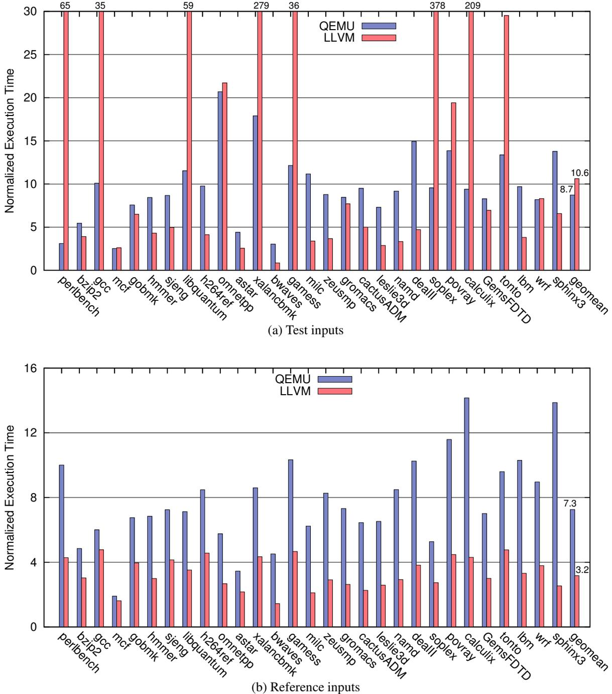
**Figure 3.1:** Comparison of QEMU and LLVM of x86 to x86-64 emulation for CPU2006 benchmarks with test and reference inputs. The results show that QEMU is suitable for emulating short-running programs and LLVM is suitable for optimizing long-running programs. Y-axis shows the normalized execution time over native run.
