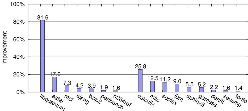
**Figure 3.12:** Improvement of trace merging with x86 to x86-64 emulation for SPEC CPU2006 with reference input. Y-axis shows the improvement rate over the emulation without trace merging.
