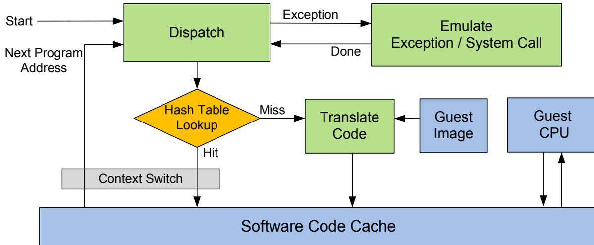
**Figure 2.1:** Control flow of the QEMU dynamic binary translator.
