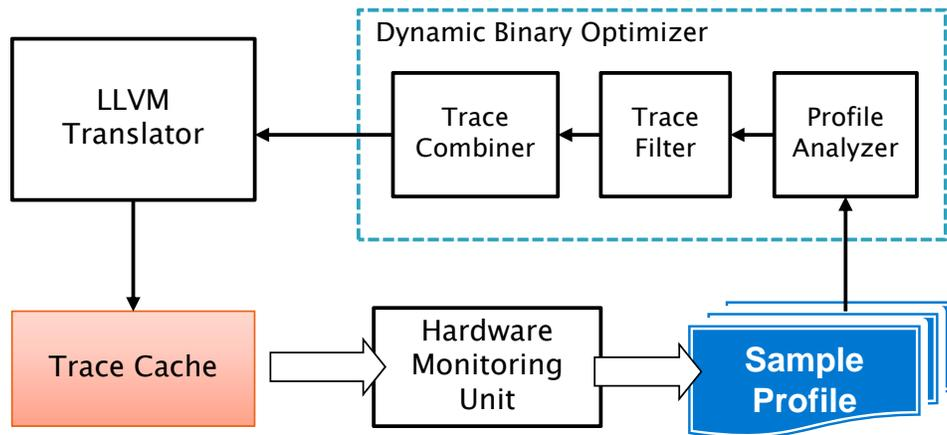
**Figure 3.5:** Workflow of the HPM-based trace merging in DBO.
