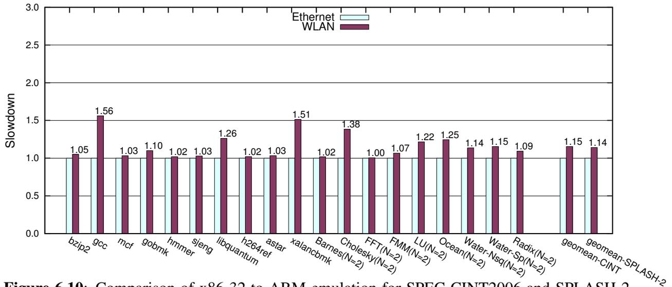
**Figure 6.10:** Comparison of x86-32 to ARM emulation for SPEC CINT2006 and SPLASH-2 benchmarks using Ethernet and WLAN. Code cache size: Unlimited.
