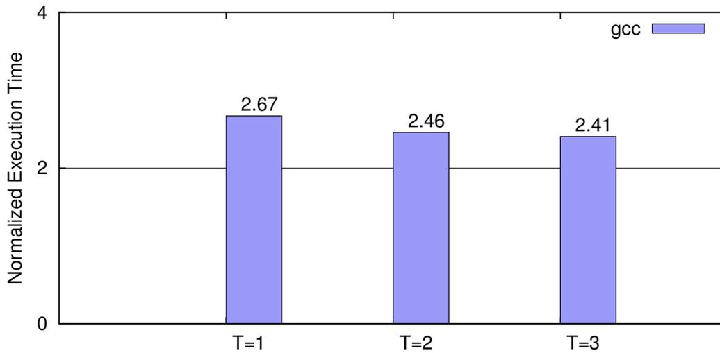
**Figure 3.13:** x86 to x86-64 emulation performance of gcc with different number of LLVM translation threads with reference inputs. X-axis shows the number of LLVM threads, and Y-axis shows the normalized execution time over native run.
