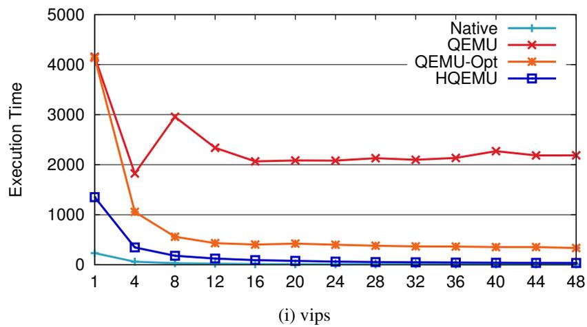
**Figure 5.4:** PARSEC results of x86 to x86-64 emulation with 32 threads and native input sets. X-axis shows the number of threads, and the unit of time for Y-axis is in seconds.
