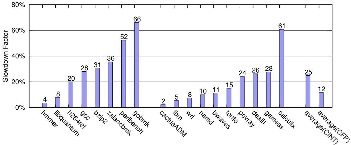
**Figure 3.15:** The slowdown factor of instrumentation-based approach over HPM sampling for trace merging.
