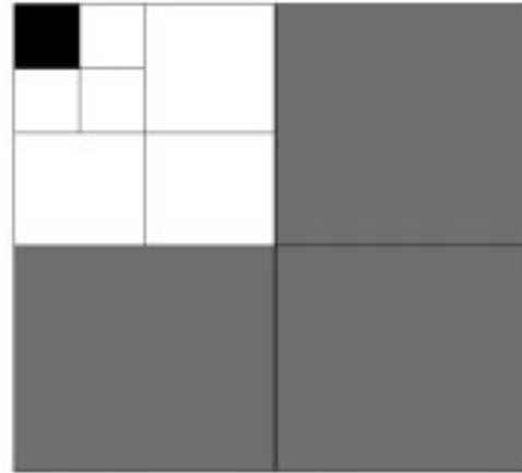
Fig. 2. Example of hiding places: A three-level wavelet decomposition with gray area indicating highest-frequency components, black area indicating lowest-frequency component, and white areas indicating the hiding places.
