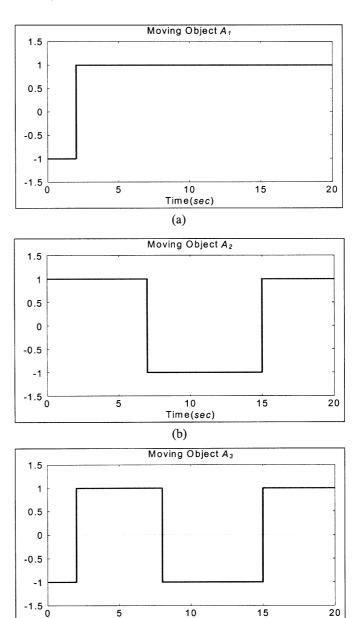
Fig. 9. The time histories of collision detection, i.e.  $sign(\cdot)$ , based on ellipsoidal bounding volume representation for all moving objects.
