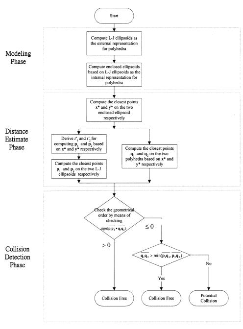
Fig. 5. Flowchart of the collision detection procedure.
