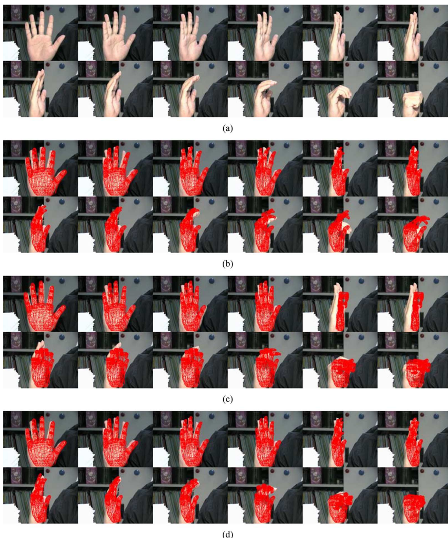
Fig. 11. Global hand motion with five-finger articulation with 22 DOFs: (a) input sequence, (b) tracking results using simple particle filtering, (c) tracking results using appearance information only, and (d) tracking results using the AGPF method.
