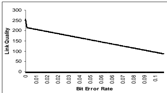
Figure 3: Link Quality vs BER for CSR chipset
