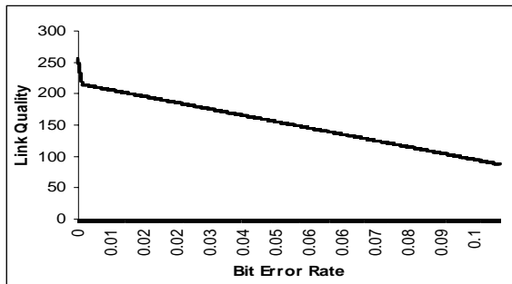
Figure 3: Link Quality vs BER for CSR chipset
