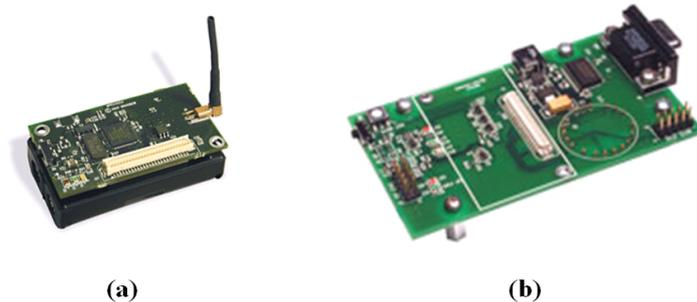
Fig. 2. (a) MICAz mote and (b) MIB510 programming board from CrossBow.
