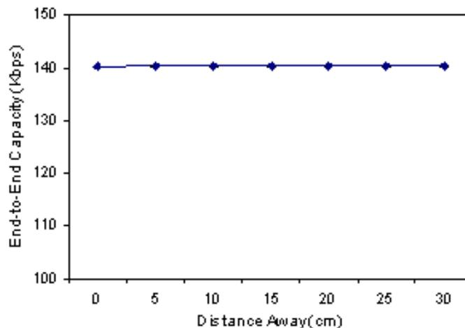
Fig. 10. SenProbe results with an interfering source at various distances.
