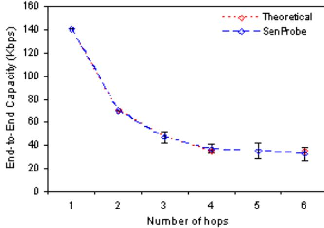
Fig. 12. SenProbe results on MICAz multihop forwarding chain testbed.
