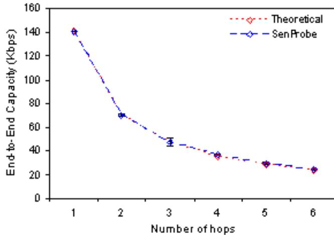
Fig. 11. SenProbe results on MICAz multihop forwarding chain testbed (within the same interfering region).
