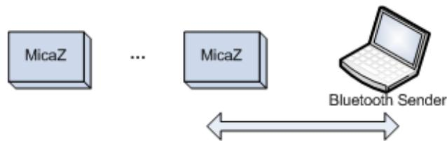
Fig. 9. Interference experiment setup, with mobile bluetooth sender is placed at various distance from the IEEE 802.15.4 receiver.
