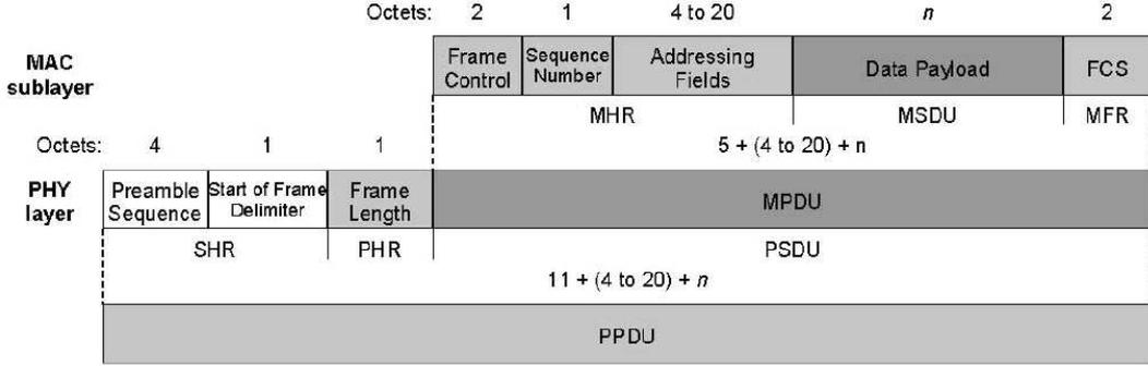
Fig. 5. Structure view of the data frame.
