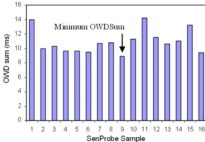
Fig. 8. SenProbe capacity estimate using the sample with minimum OWD sum.
