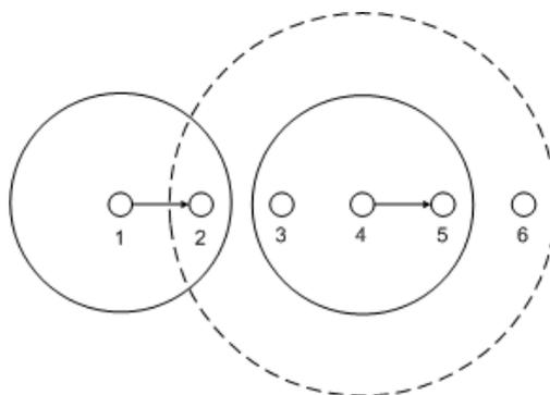
Fig. 3. The chain topology, where the solid-line circle denotes a node's effective transmission range and the dotted-line circle denotes a node's interference range.
