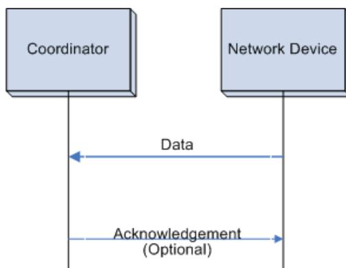
Fig. 4. Communication to a coordinator in a nonbeacon-enabled network.
