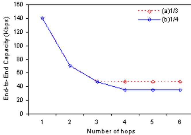
Fig. 6. Theoretical capacity in an ideal adhoc multihop forwarding chain. (a) denotes the path capacity when interference range is equivalent to the transmission range. (b) depicts the path capacity when interference range is twice of transmission range
