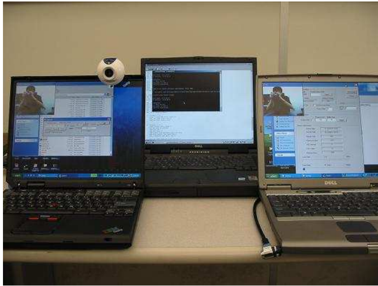
Fig. 10. Hybrid testbed consisting of three laptops: video server, Ns-2 simulation workstation, and video client (from left to right).
