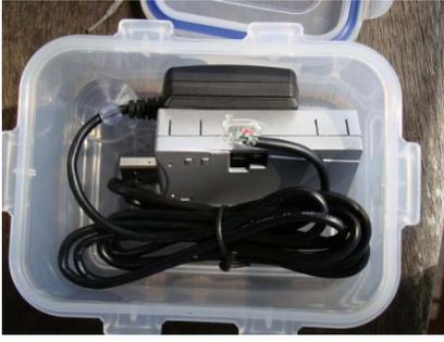
Fig. 6. The EcoNet client device packed in a LOCK&LOCK box
