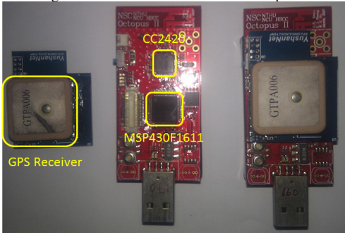
Fig. 8. GPS extension board and Octopus mote
