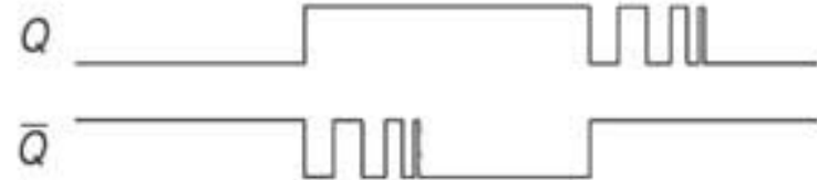
d. Effect of contact bounce
