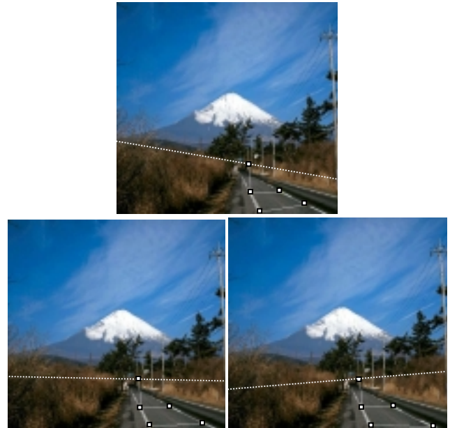
Figure 4 Different auxiliary lines (in which the fifth control point P_5 should be lying on) generated by dragging the control point P_4 to different image positions. The control points of concave type are used in this example.
