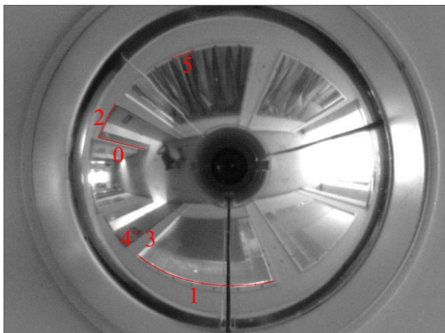
Figure 4. The lines used for the length-ratio results, where line 0 is the unit length.
