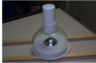
Figure 8. The omnidirectional camera used in our experiment, which is non-perspective.
