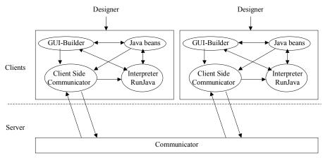
Figure 2. The i-Code system architecture.
