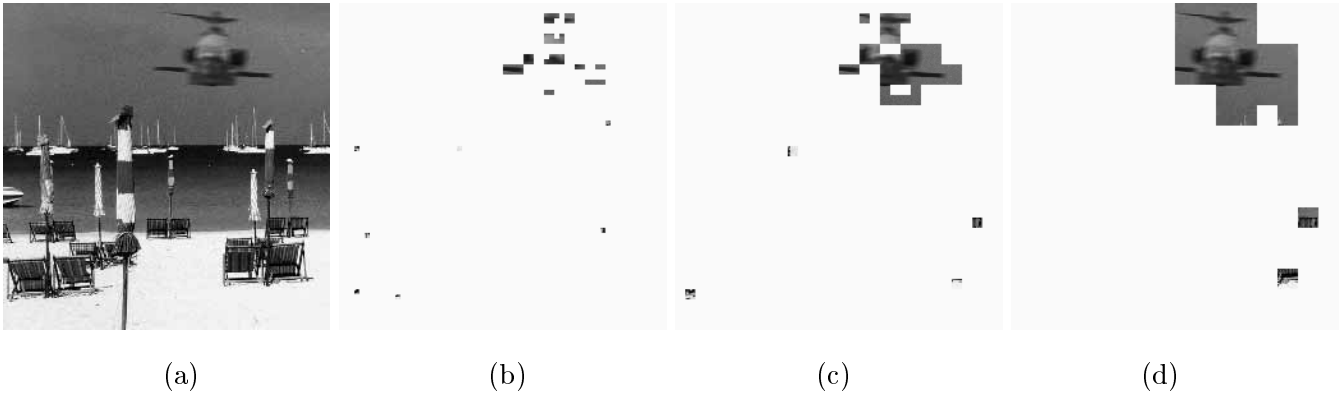
Figure 7: Malicious manipulations of non- SDS areas: (a) maliciously tampered with image with a “helicopter” in the sky; (b)~(d) detected results of (a) at 2^2 \sim 2^4 scales when \sigma = 128 .
