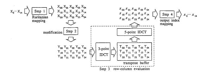
Fig. 2. One 3-point IDCT component, one transpose buffer, and one 5-point IDCT component are necessary for computing the row-column evaluation for the 15-point prime-factor IDCT.
