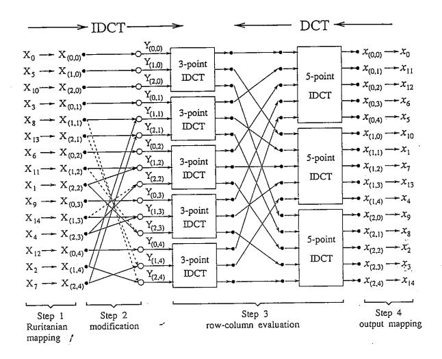
Fig. 1. The signal-flow graph for implementing the 15-point IDCT, which can be decomposed into the  $(3 \times 5)$ -point 2-D IDCT. If signals flow from left to right, it performs the IDCT; if signals flow from right to left, it performs the DCT. Solid lines represent transfer factor 1, while dashed lines represent transfer factor -1. Circles  $\circ$  represent adders.
