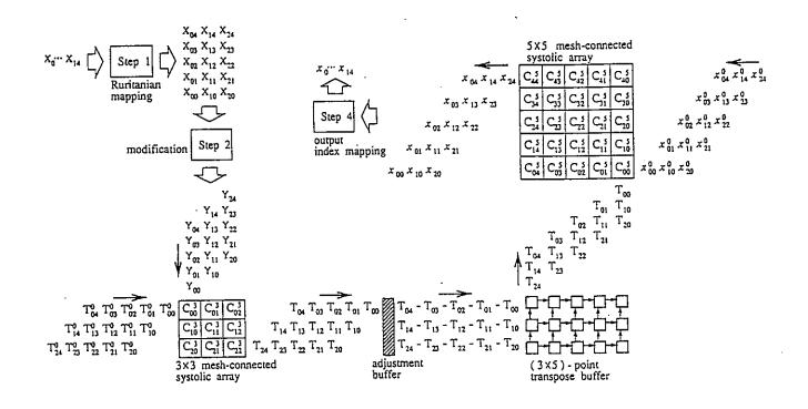
Fig. 3. The complete data-flow diagram of the mesh-connected systolic array implementation for computing the 15-point prime-factor IDCT.
