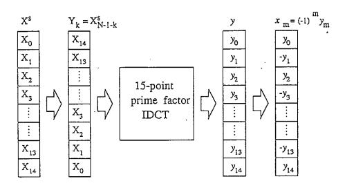
Fig. 5. The procedure for computing the 15-point prime-factor IDST from the 15-point prime-factor IDCT.
