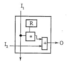
Fig. 4. Each processing element of the mesh-connected systolic array contains a multiply-and-add circuit, which implements  $O = I_2 + R * I_1$ .
