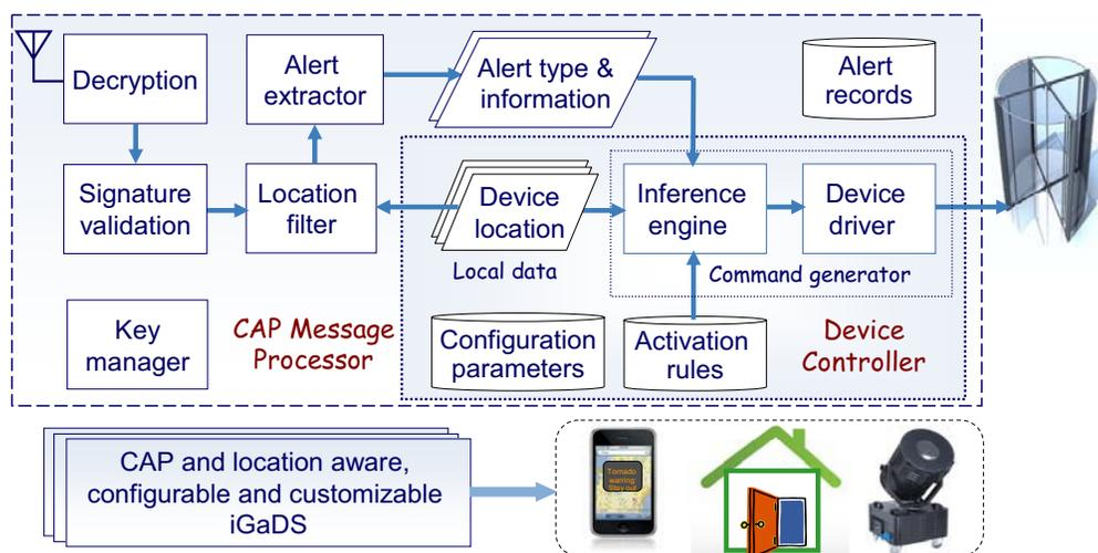
**Figure 3 General structure of embedded iGaD**
