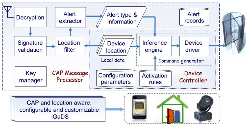
**Figure 3 General structure of embedded iGaD**
