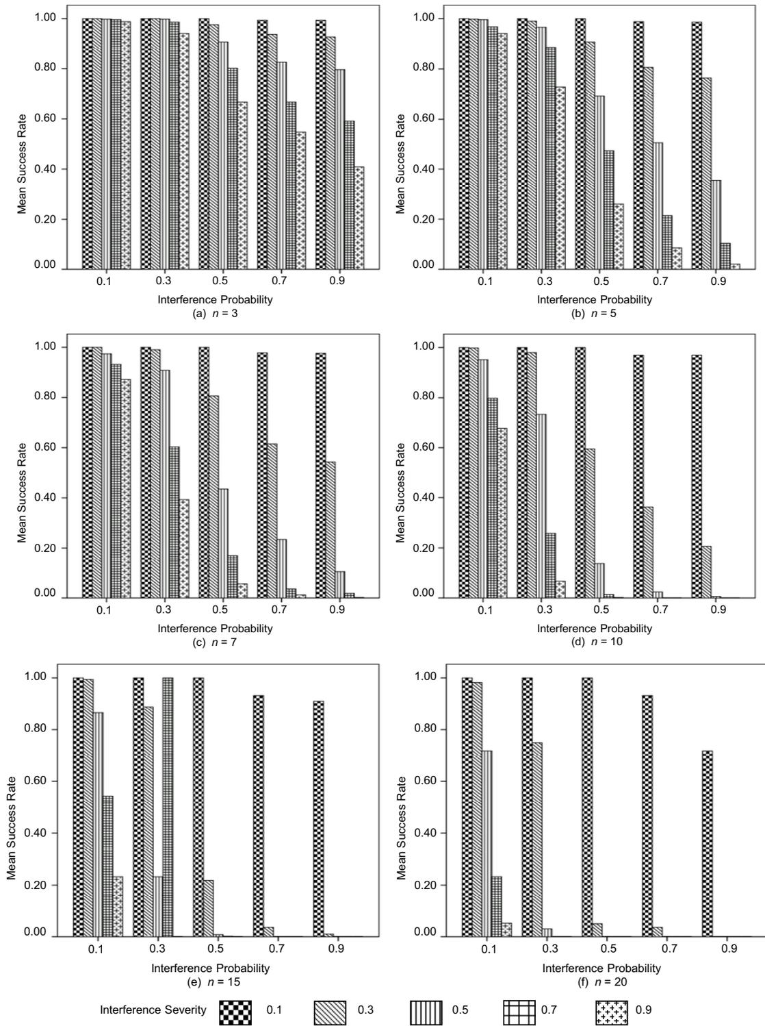
Figure 10 Success rate of advanced OMAT\_MVF algorithm as function of interference parameters
