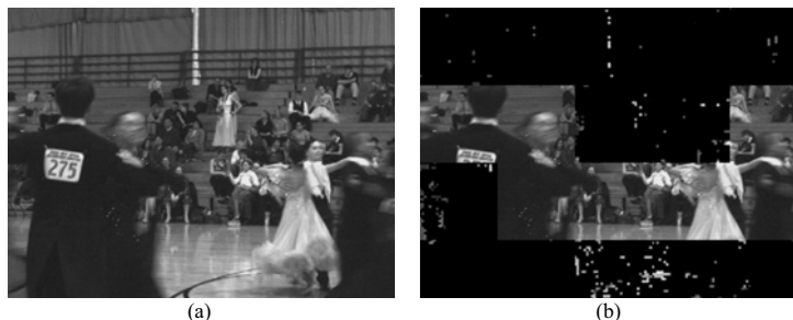
Fig. 7. (a) The original key frame K_{I,48} to be re-encoded in Fig. 6 and (b) the spatial display of its significant wavelet coefficients with some blocks with intra mode.
