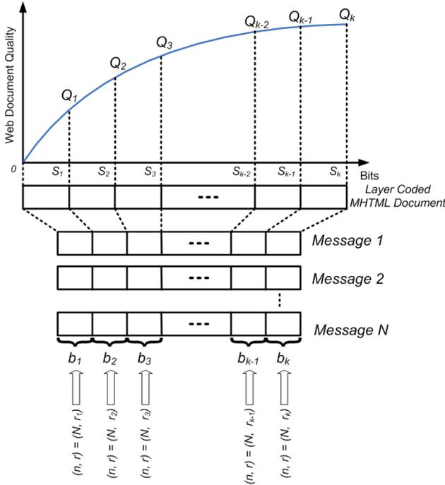
Fig. 2. Illustration of the Layered MDC scheme with unequal erasure protection. Each web document is encoded into  $k$  quality levels using layered coding. The  $i$ -th quality level content is erasure protected with replication factor  $r_i$  and split equally among  $N$  relays ( $r_1 > r_2 > \dots > r_{k-1} > r_k$  and  $N \geq k$ ).
