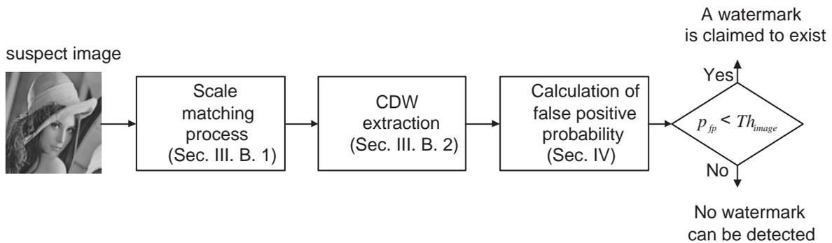
Fig. 4. Block diagram of the process of determining the existence of a watermark.
