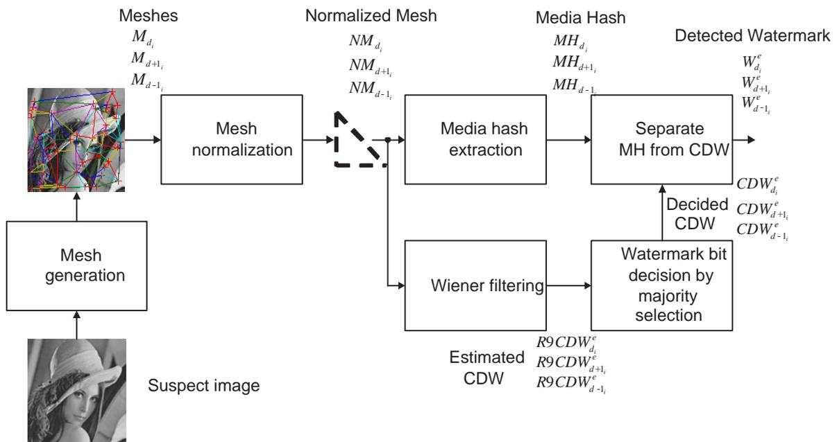
Fig. 5. Block diagram of the CDW extraction process.
