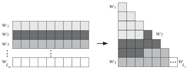
Fig. 2. (left) The repeated watermark bits (each bit is repeated 9 times) are arranged and embedded in a normalized mesh (right).
