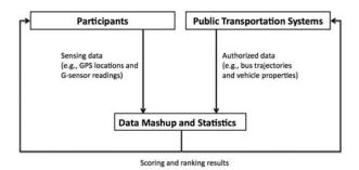
Figure 1: The architecture of the CMS system
