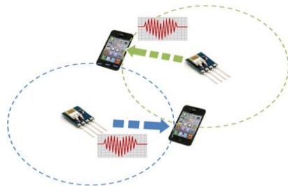
Fig. 1. The co-located BANs may suffer from inter-BAN interference if they operate in the same channel.
