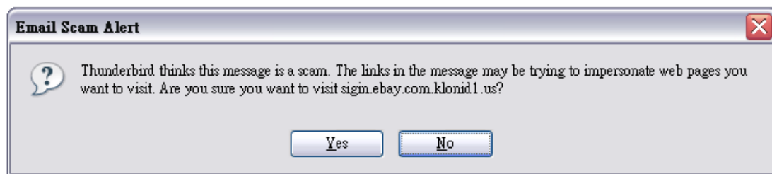
Figure 8 The second warning interface of Thunderbird Phish Detector. It pops up a warning dialog if the user clicks on the link in the possible scam email (in Figure 7).
