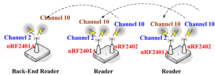
Fig. 6. Demonstration of multi-hop relaying.
