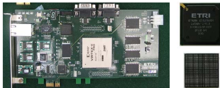
Fig. 8. The LATONA card and ASIC.
